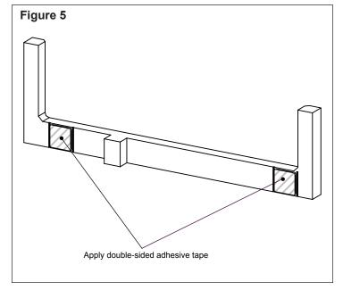
Locate and position the installation jig. Clean the area where FridgiGuard will be installed with alcohol. Position the jig as shown with FridgiGuard against the refrigerator body. Press and hold the jig until the double-sided tape adheres. See Figure 6.
